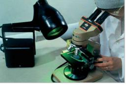
B-100Y and B-100YP produce high contrast light for fine surface particle detection.
