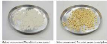
(Before measurement) The white rice was spread evenly over the pan. (After measurement) The entire sample turned yellow.
