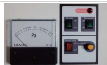
Pirani Vacuum Gauge and Control Panel
